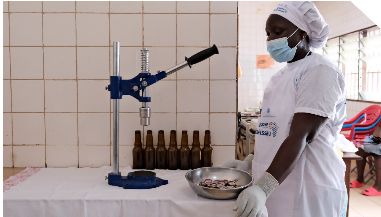
Maria Sambú, from the Azedinha Group Cooperative, using the Manual Crown Bottle Capping Machine from the field laboratory and food processing equipment delivered to 33 Conformity Assessment Bodies and Agents of the Mango Value Chain
