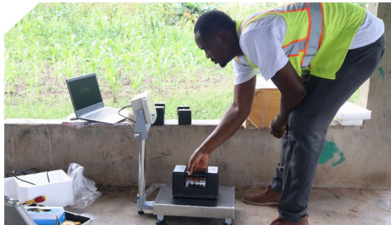
UNIDO WACOMP-GM trained TGSB Metrologist, Abdoulie F. Njie, calibrating precision weighing scales supplied by the project at a vegetable garden
