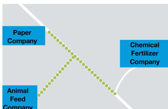
Figure 2: Length of steam from Paper Company to connect to steam system of the other companies is 600 meters
